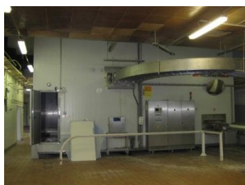
Spiral freezer MECATHERM
