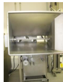
Soft Separator / Desinewing BAADER
