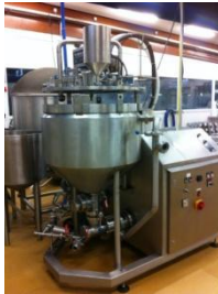
Emulsification-Homogenization Machine BALIK
